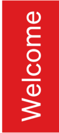
SIGN 7: WELCOME SIGNAGE 1800 w x 800mm h Vinyl cut graphics applied to prefinished red ACM
