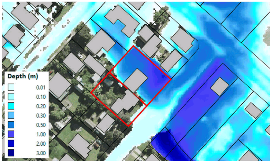
Plate 1 1%AEP flood depths under existing conditions.
