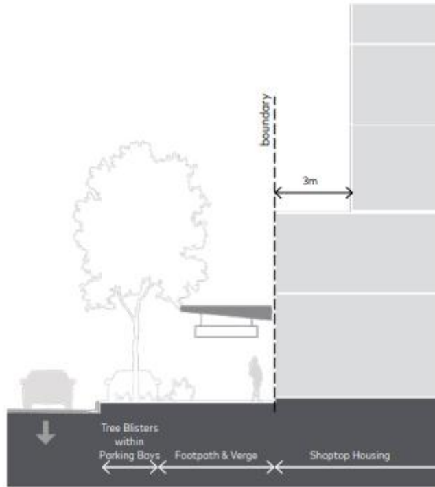
Figure 7.5 – Main Street Section – Non-Residential Interface
